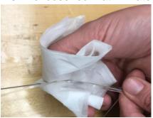
**2.7** Repeat the process until all remaining material has been removed from the individual fibers. Two or three passes should remove the matrix from the fibers.
