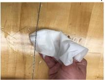
**2.4** Allow the fibers to soak in the alcohol for at least five minutes. The matrix material will begin to loosen.
